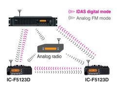
The IC-F5123D series can receive both analog mode and digital mode signals on a single channel and automatically selects the received mode to reply to the received call, while the talk back timer remains. It's a smart way to grow into digital radio – at your own pace, as your budget and comfort allow.
