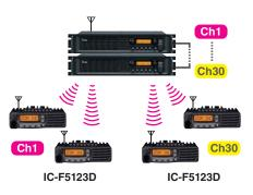
The IC-F5123D series can be used in an IDAS single-site trunking system.
