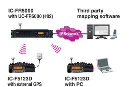
When used with an external GPS receiver, the IC-F5123D series can transmit accurate position data for use with vehicle management applications.
